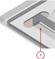
Figure 15: Replacing the Silicone Rubber of the Silicone Holders
