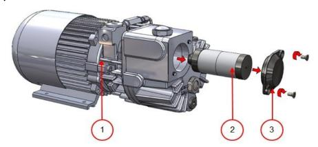
Figure 11: Replacing the Oil Exhaust Filter (Pump 8 m3)
