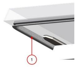
Figure 16: Replacing the Lid Gasket
