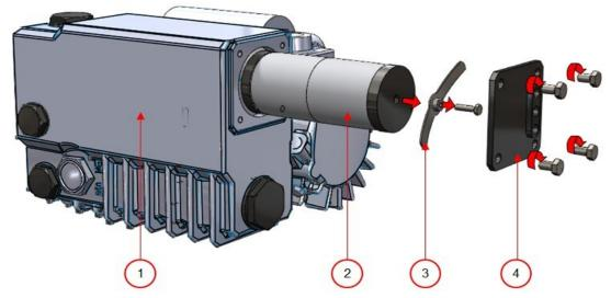
Figure 12: Replacing the Oil Exhaust Filter (Pump 16 m3)
