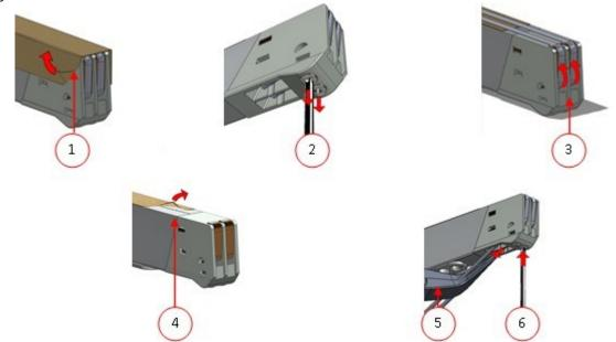
Figure 14: Replacing the Sealing Wire
